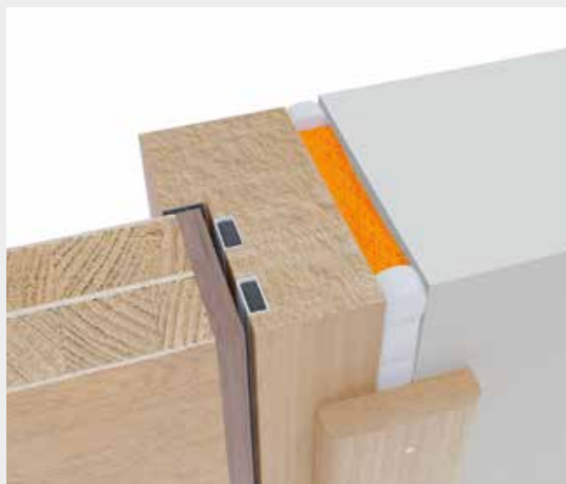
FAS Fire Door Silicone Sealant with FAS Fire Door Foam™ for joint widths up to 30mm to achieve fire ratings of up to 60 minutes when applied correctly.
