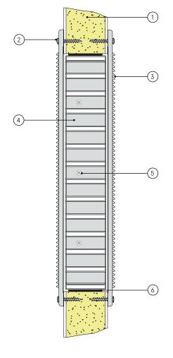
Note: Screw holes based on 600mm square grille. Location and number may vary depending on the size of the grille. Max centres 200mm.
