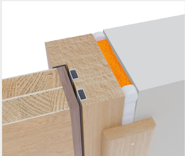
Image B – FAS Fire Door Intumescent Acrylic Sealant with Fire Door Foam™ for joint widths up to 35mm to achieve ratings of up to 120 minutes when applied correctly.
