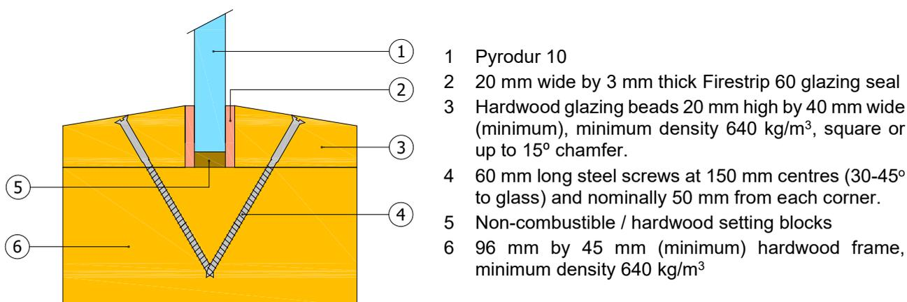
This Certificate of Approval relates to the sizes of Pyrodur 10 glass shown in Table 13 below, when used in conjunction with the above system.
