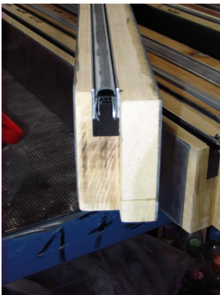
Fig. 4 Photo of the door section with floor seal (taken by ift Laboratory for Building Acoustics)
